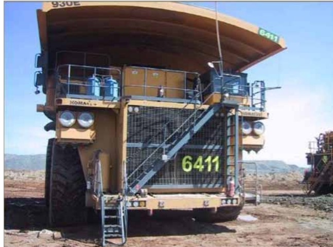
Figure 2: A mining truck showing access to the driver cabin (Courtesy of BHP Billiton)
