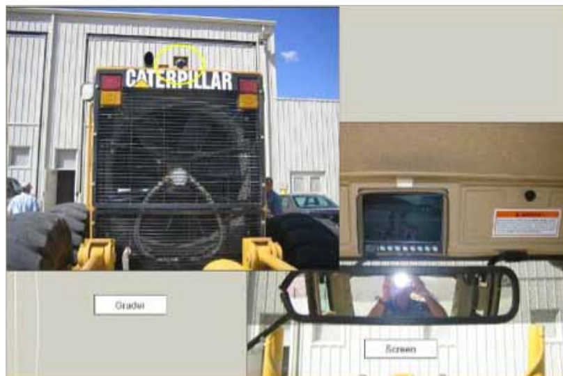
Figure 4: Rear camera system installed on a grader (Courtesy of BHP Billiton)
