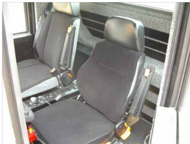
Figure 3: Operator's cabin designed to improve seating (Courtesy of Rio Tinto)
