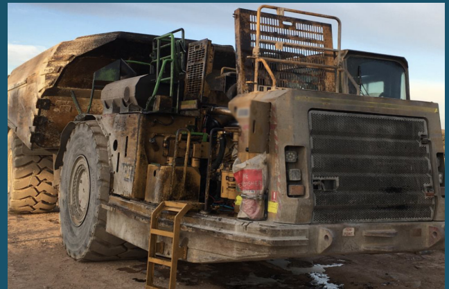
Dump truck travelling out of the underground caught fire as a result of engine bay covered in hydraulic oil. New South Wales Resources Regulator Fires on Mobile Plant, October to December 2020.
