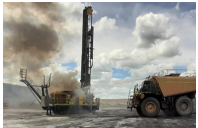
Drill rig catches fire. Image sourced from Resources Safety and Health Queensland.
