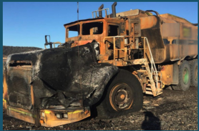
Watercart extensively damaged following drive shaft failure. New South Wales Resources Regulator Safety Bulletin November 2019.
