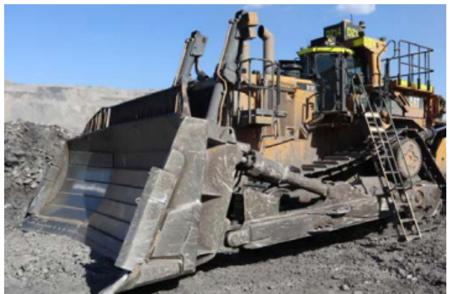
Oil made contact with hot surfaces of exhaust/ turbo components and ignited. New South Wales Resources Regulator Fires on Mobile Plant, January to March 2019.
