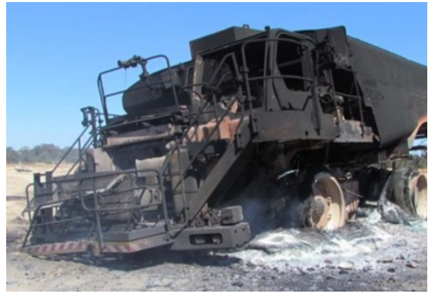
Water truck totally destroyed by fire at an open cut coal mine. New South Wales Energy Mine Safety, Alert No SA15-05.
