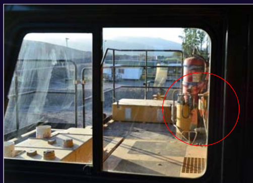
Visibility restriction associated with poorly positioned fire suppression tanks
