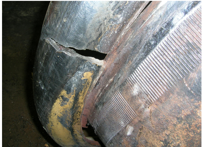
Photograph 1: Fatigue damage of rim and rim components, if not detected, such as this flange ring can have catastrophic consequences.
