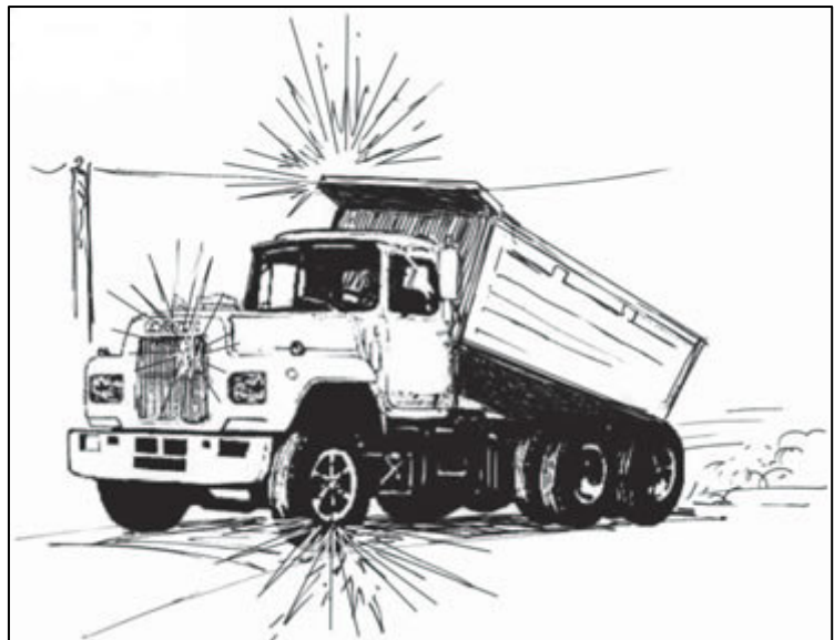
Accidental contact with overhead powerlines, or electrification by lightning strike is known to cause pyrolysis and subsequent violent explosion of in some or all vehicle tyres. This hazard can be best eliminated by designing roads away from powerlines. (sketch from [31])
