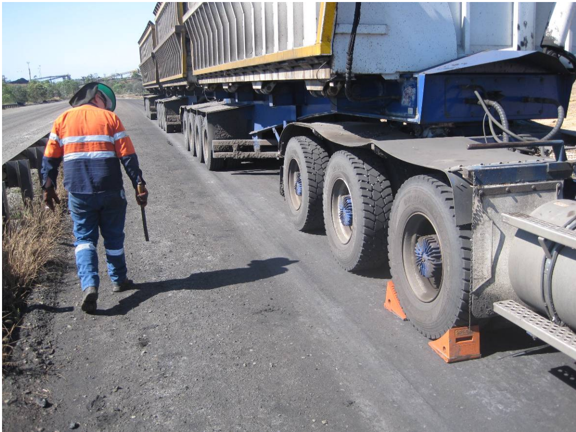
Figure 37 – Vehicle, tyre and rim checking station - note the use of the wheel chocks.
