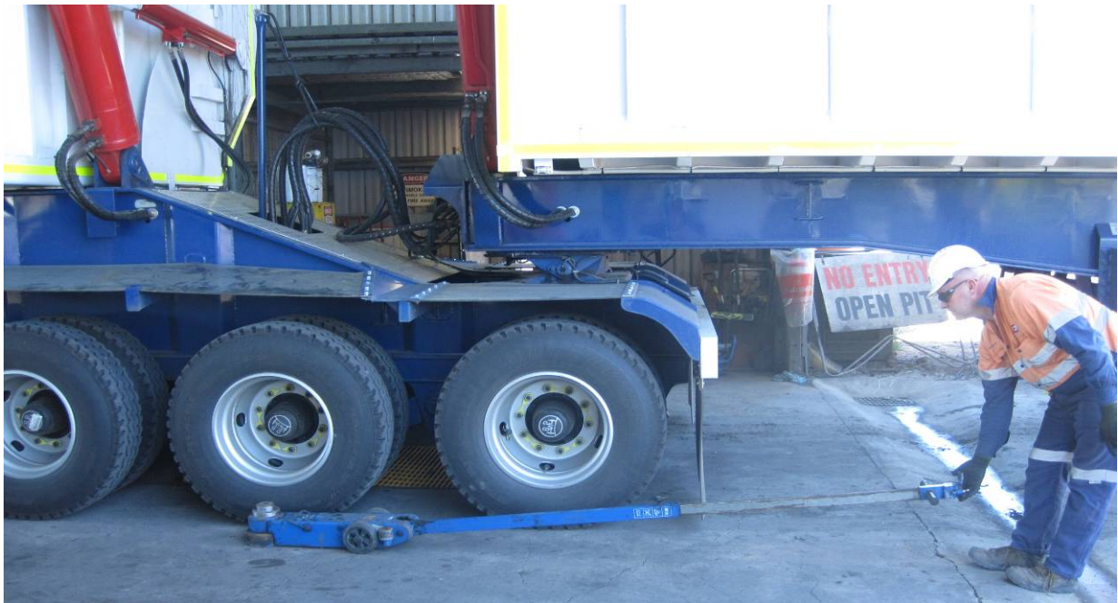
Figure 20 - Extendable trolley jack, there are no manual task issues with safely placing the jack under the vehicle compared to the previous scenario
