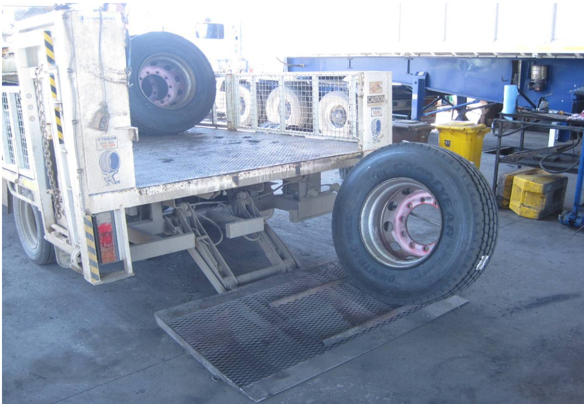
Figure 15 – Tailgate designed to lift/lower tyres and wheel assemblies onto service vehicle reducing manual handling
