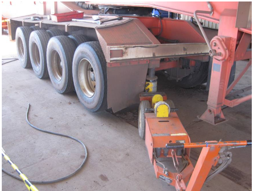
Figure 21 – The axle is raised off the ground by supporting the bogey chassis. Note: this should only be done if the OEM nominates the chassis as a safe lifting/support point.
