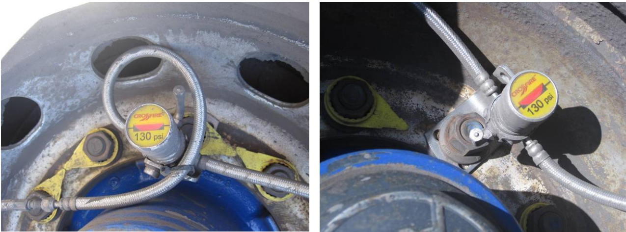
Figure 26– on wheel pressure monitoring system
