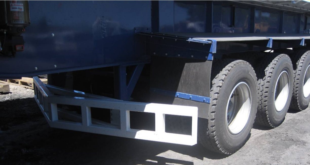
Figure 7 - 'Cowcatcher' on coal haulage trailer
