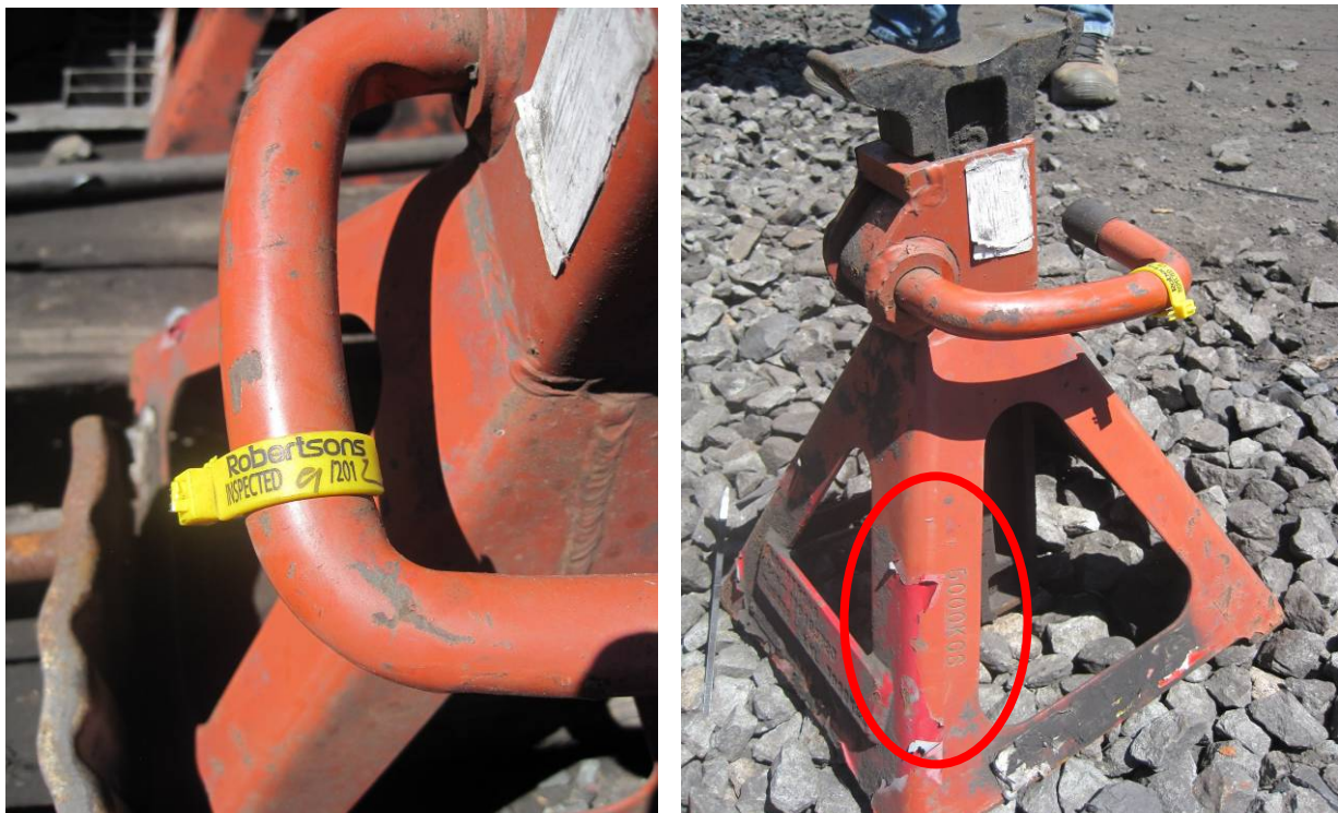
Figure 18 – Engineered and tested vehicle stands, note the SWL on the stand
