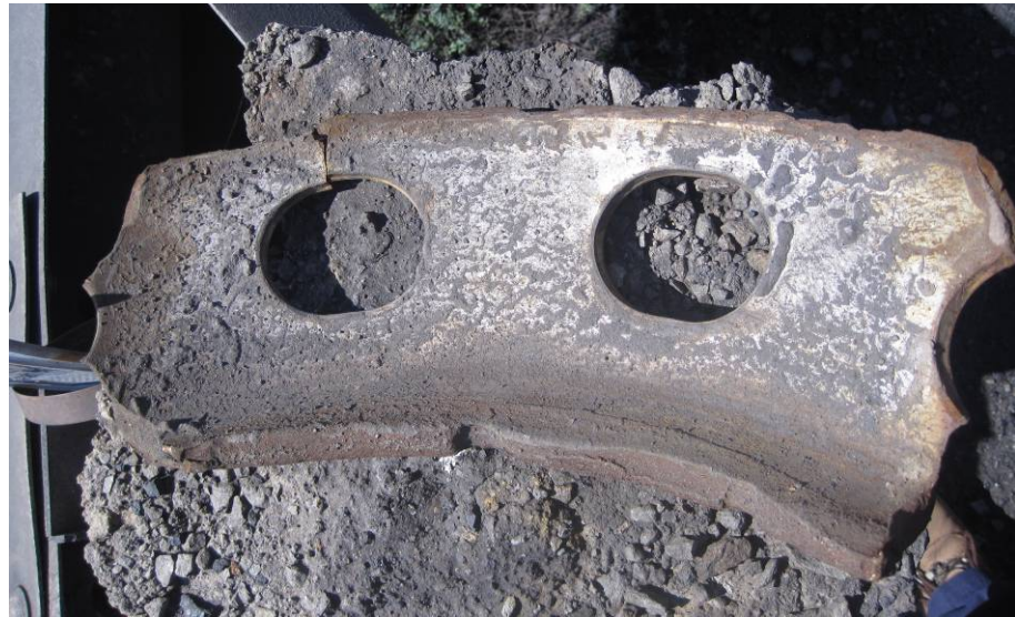
Figure 32 – Piece of shrapnel from a disintegrating wheel or rim
