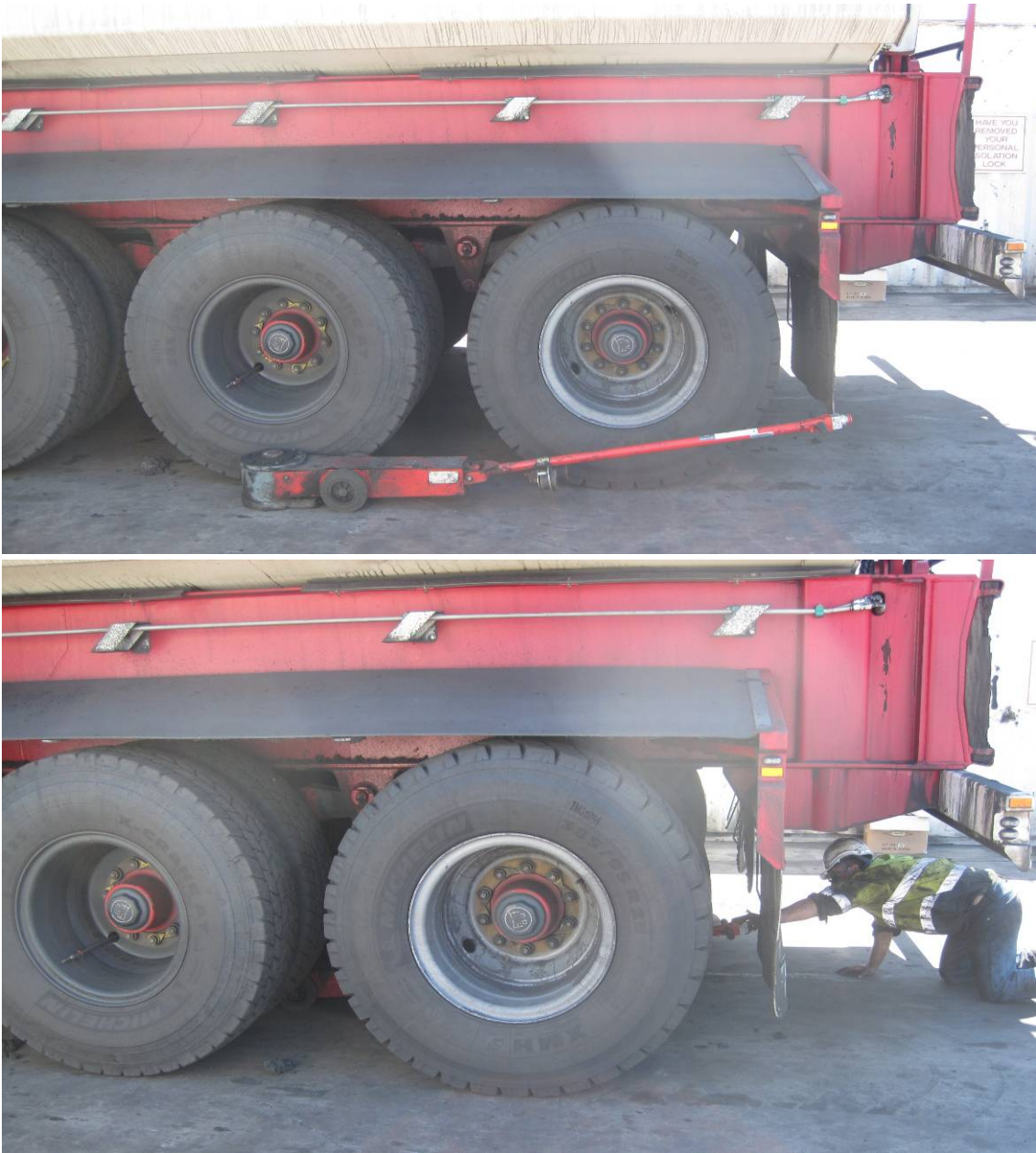
Figure 19 – Trolley jack – note the difficulty with placement under the vehicle
