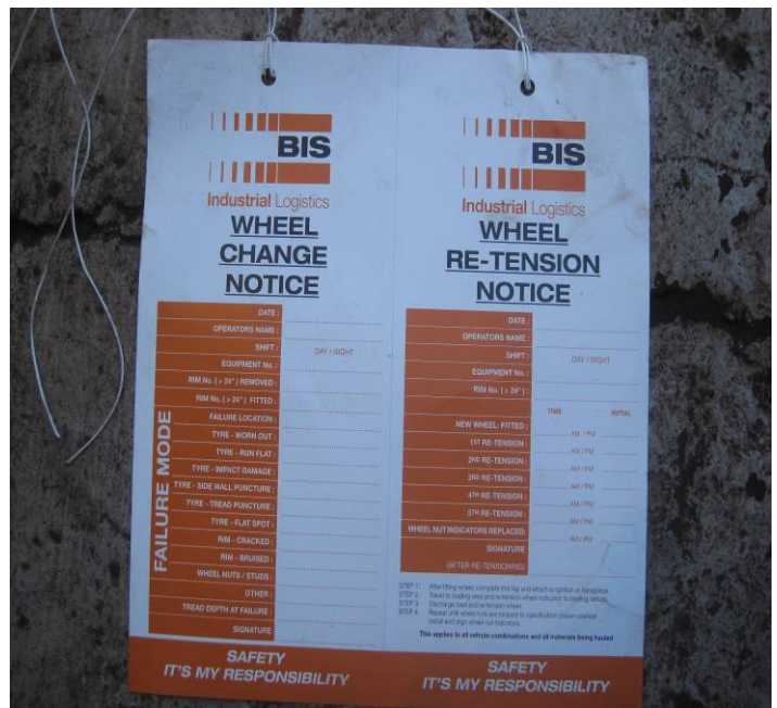
Figure 9 – Typical tyre maintenance tags including retention tag
