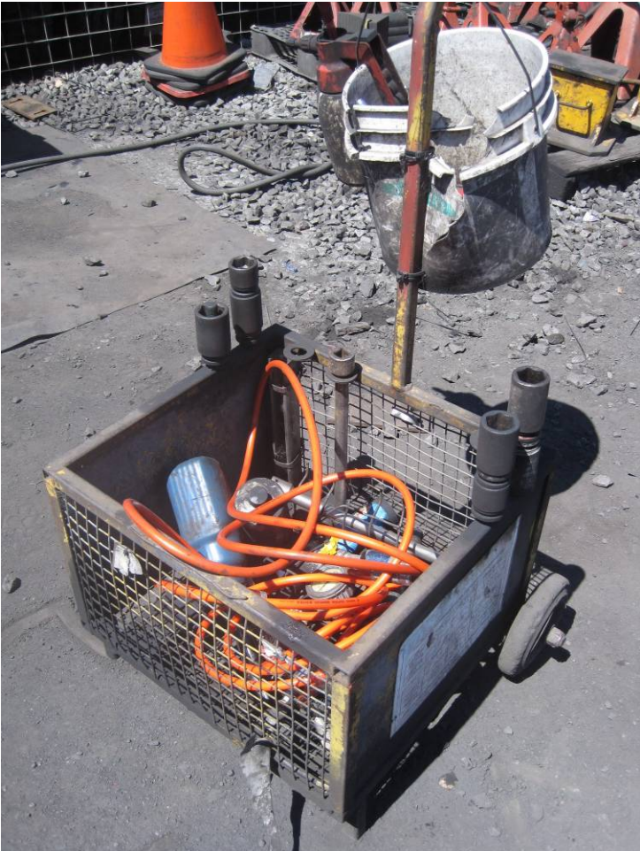
Figure 10 – Trolley holding tyre maintenance tooling, note the torque chart attached to side of trolley
