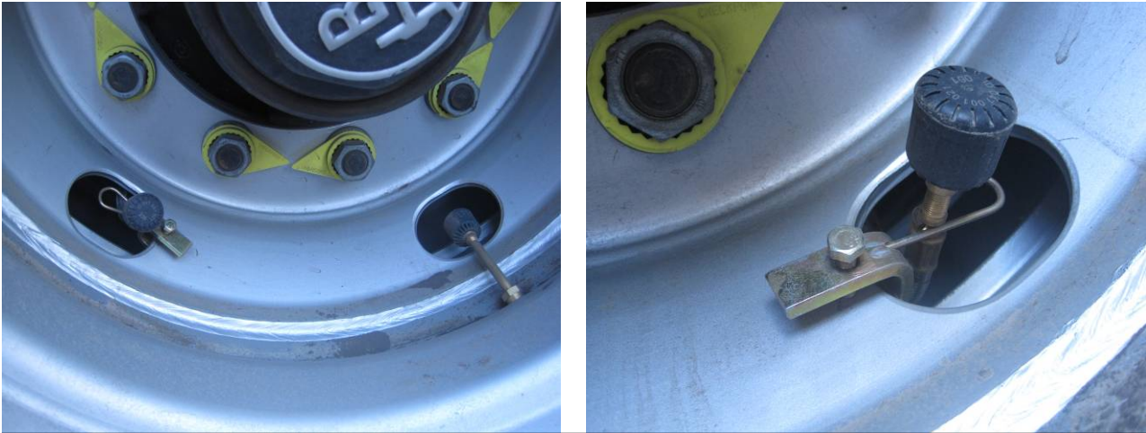
Figure 27 - Automated pressure monitoring system, and valve stem securing system
