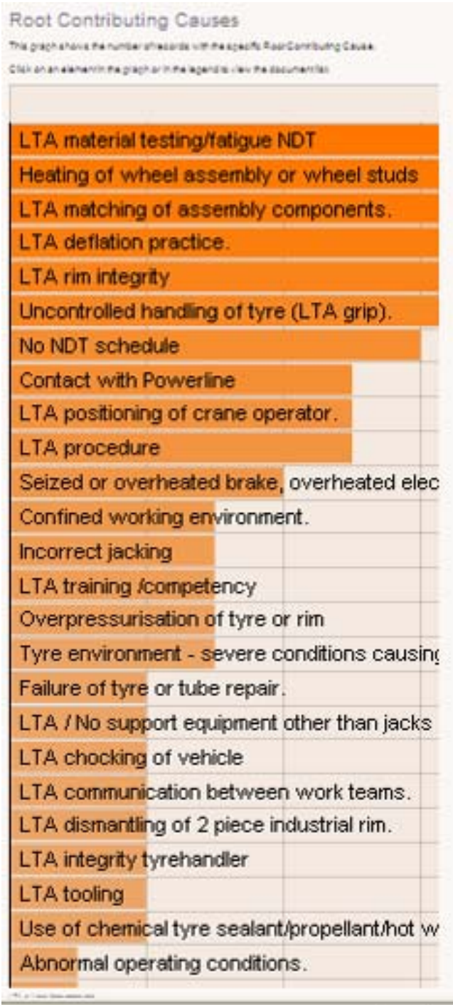
Figure 3 – Root causes for tyre and rim related incidents and accidents (refer to Tyregate for more information)
