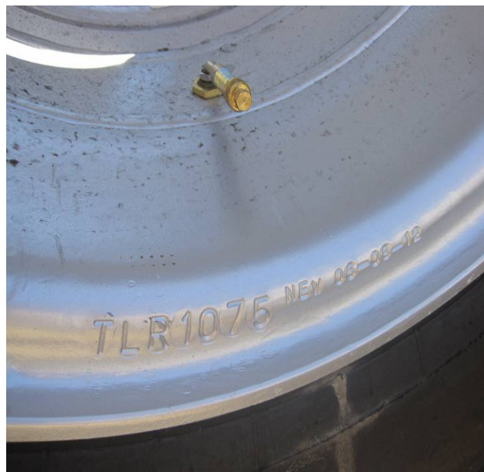
Figure 30 – Unique rim identification number on a non-earthmoving wheel
