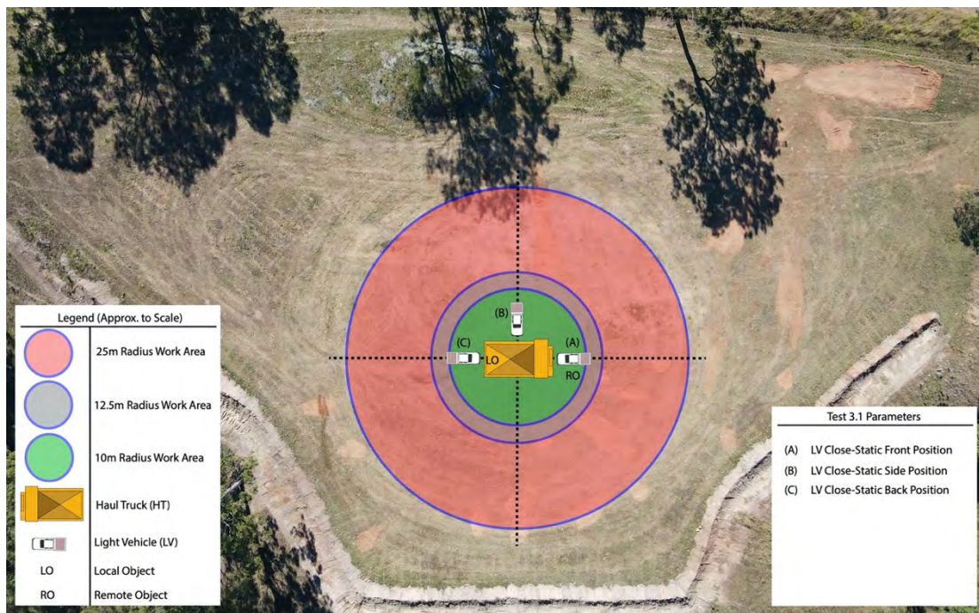
Figure 6: An overhead representation of Test 3.1, represented at the Mining3 Test Facility. Please note that all object and work areas are done approximately to scale to provide an indication of size.
