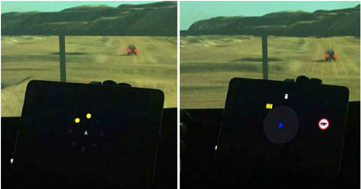
Figure. 50: Ring (left) and Schematic (right) interfaces indicating the presence of another truck (unseen) and a stationary light vehicle.
