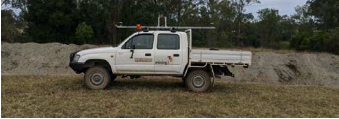
Figure. 14: LV instrumented with the sensor bracket containing the dual antenna GNSS system, stereo camera and LIDAR.
