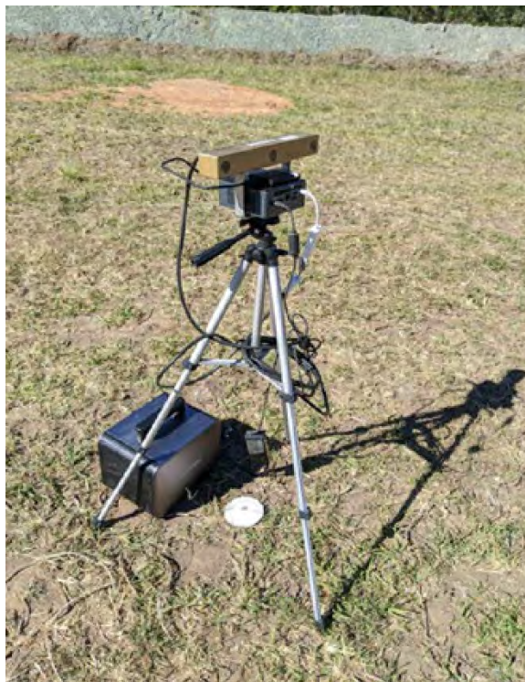
Figure. 15: Bystander DAQ system including the battery, mini-computer and stereo camera located within the test pad
