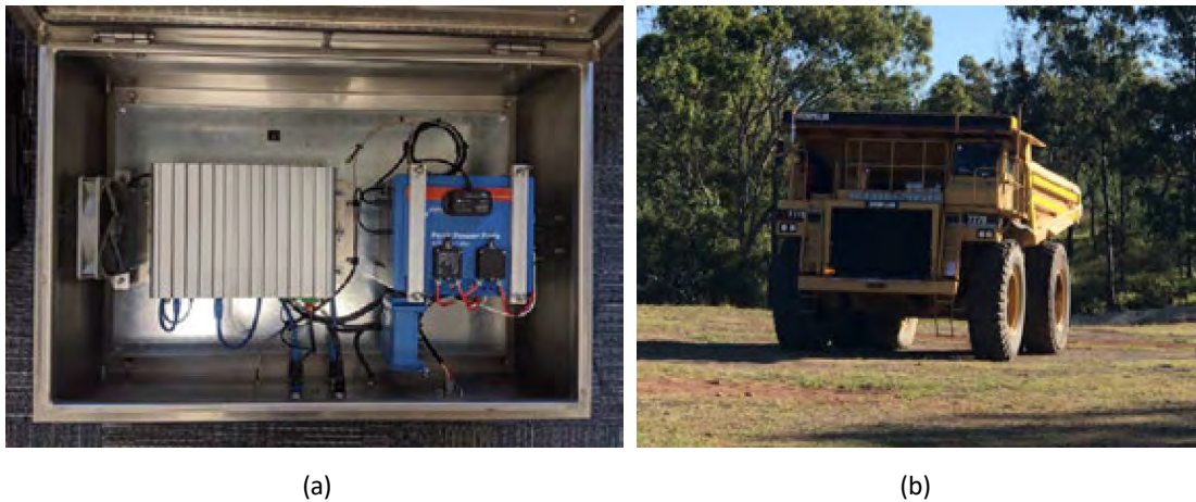
Figure. 13: HT DAQ system including the: (a) data logging box; and (b) haul truck equipped with the dual antenna Global Navigation Satellite System (GNSS) unit.
