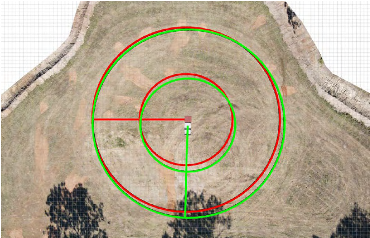
Figure. 23: Illustration of the use of the visualisation tool to position the LV between test activities. The green target represents the position and orientation of the LV and the red target represents the position and orientation of the required test location.
