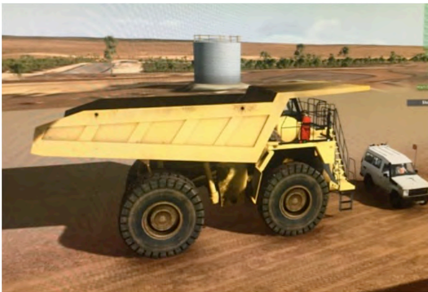
Figure 3: A simulation of a stationary light vehicle located in front of a stationary haul truck. The view from the operators seat (lower panel) includes visibility of the light vehicle flag in the bottom right of the windscreen.
