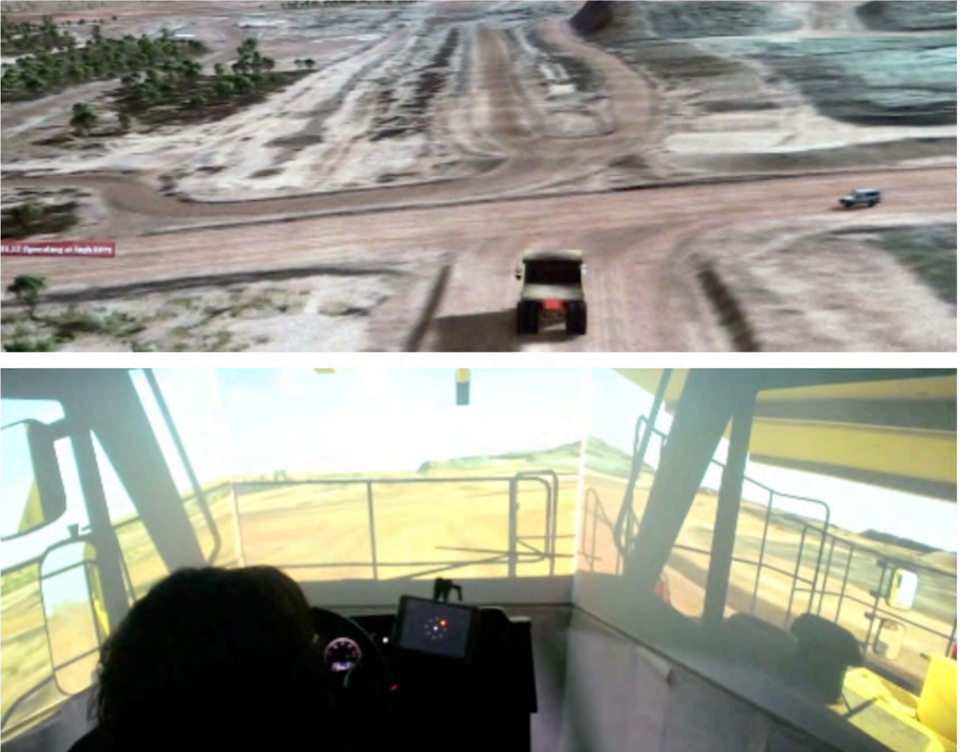
Figure 2: Still taken from a simulation trial conducted as part of ACARP project C24028 in which an approaching light vehicle is continuously obscured behind the A pillar of a haul truck cab as the vehicle approach a T intersection. In some situations, visibility restrictions prevent an operator from perceiving presence of another vehicle through direct vision alone. In this trial, an interface being trialled alerted the participant to the light vehicle's presence and braking was initiated prior to the light vehicle being visible.
