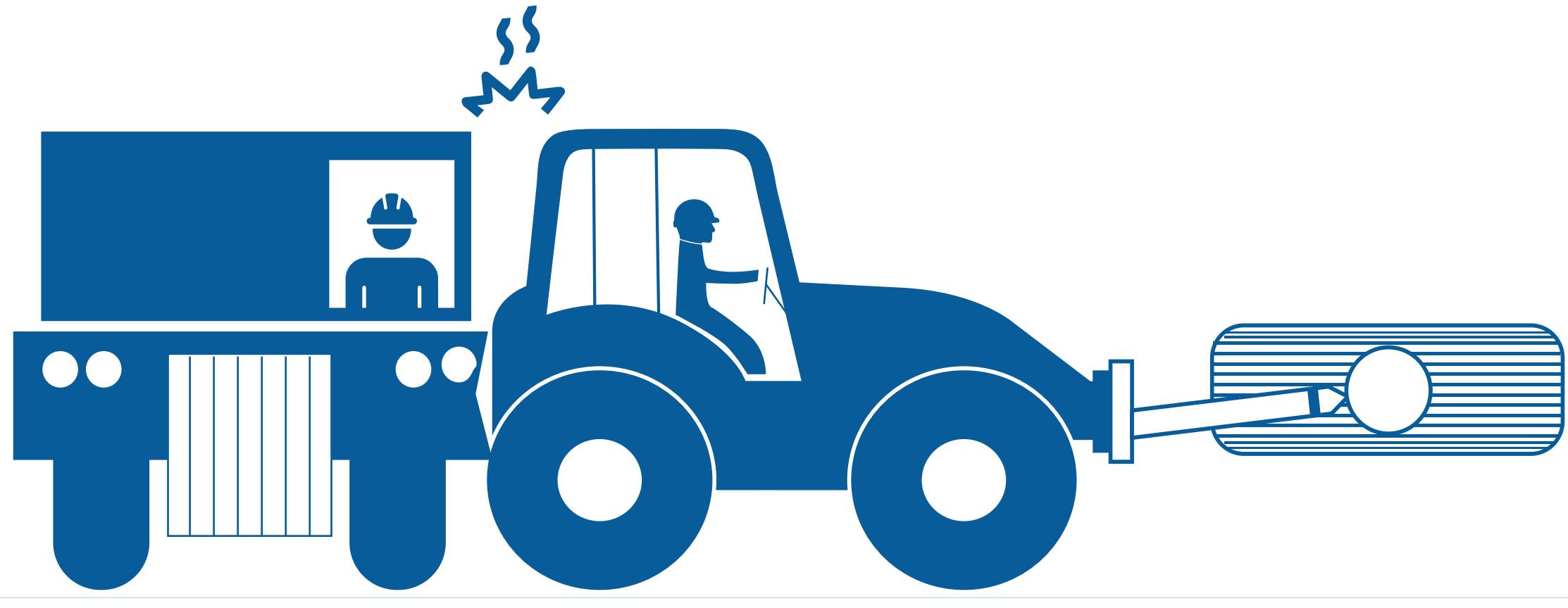
Tyre handler collides with haul truck or equipment at rear when reversing
