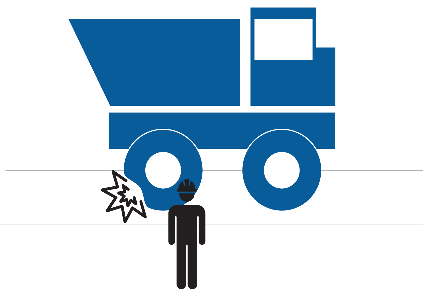
Air blast or projected tyre/wheel/rim component strikes fitter – within line-of-fire
