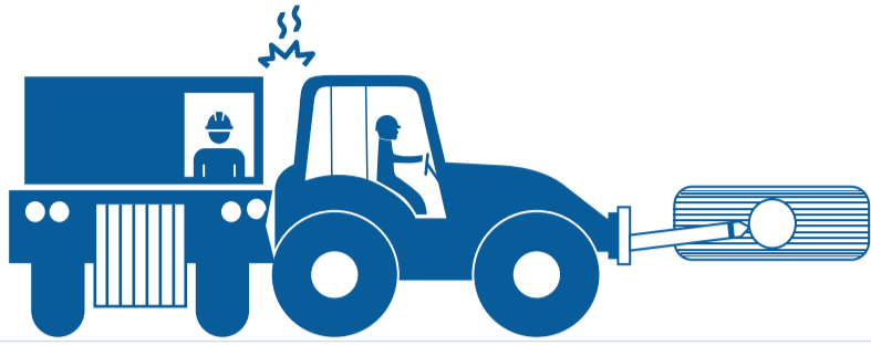
Tyre handler collides with haul truck or equipment at rear when reversing
